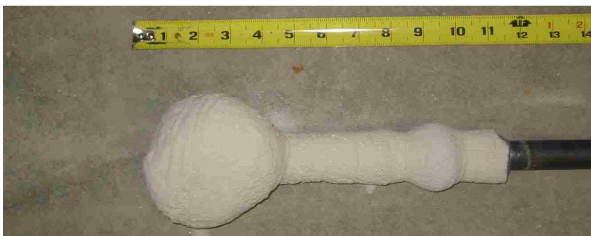
Figure 4.27. Photograph of Exhumed Pile 2B Bond Zone
