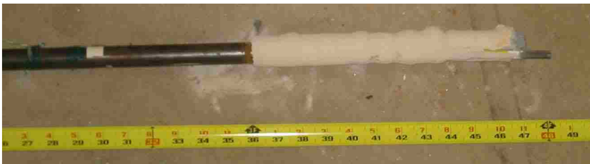
Figure 4.24. Photograph of Exhumed Pile 1F Bond Zone
