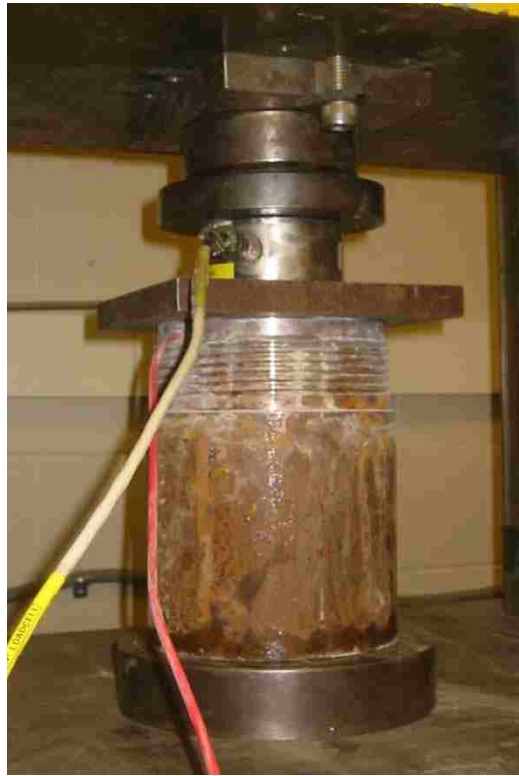
Figure 5.14. Photograph of Mock Section of Micropile for Strain Gage Calibration
