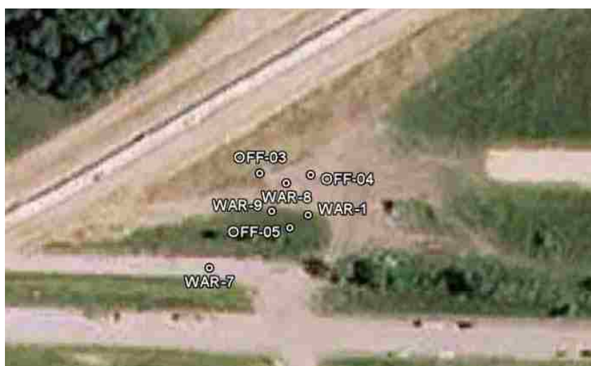
Figure 5.3. Warrensburg Test Site Boring Locations [Likos et. al. 2011]
