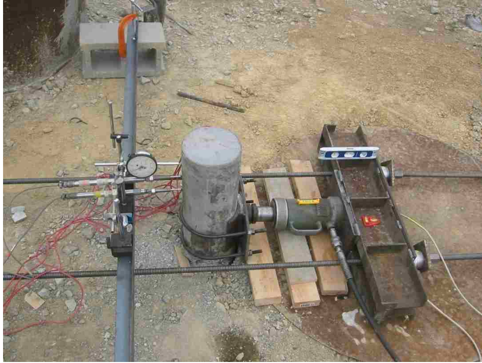
Figure 5.24. Lateral Load Test
