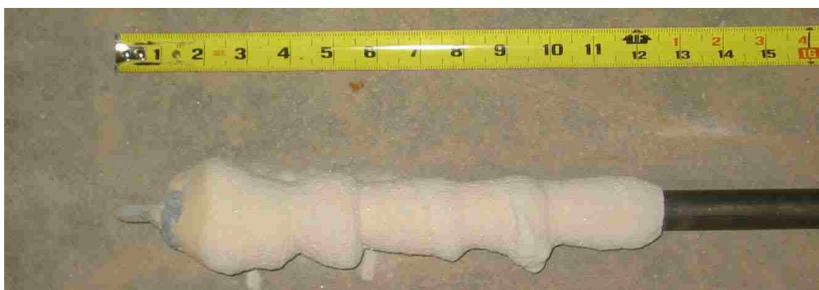
Figure 4.26. Photograph of Exhumed Pile 2F Bond Zone
