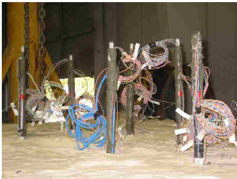
Figure 4.23. Photograph of Completed Model Micropiles with Central Bar (Step 6)
