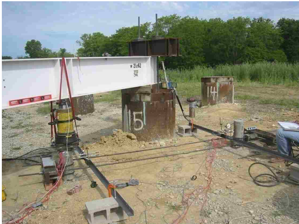
Figure 5.25. Simultaneous Lateral and Combined Load Tests
