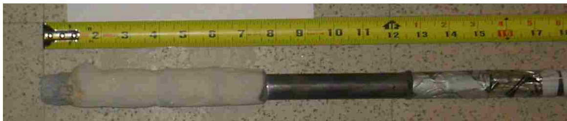
Figure 4.28. Photograph of Exhumed Pile 3D Bond Zone
