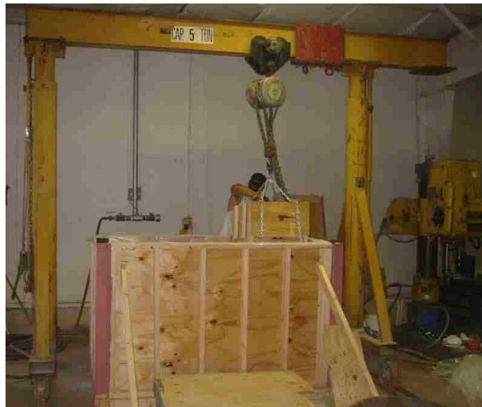
Figure 4.10. Photograph of Sand Placement Showing Pluviator and Gantry Crane
